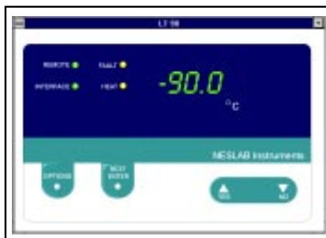
View a virtual controller screen which allows remote monitoring and operation of product control panel.
