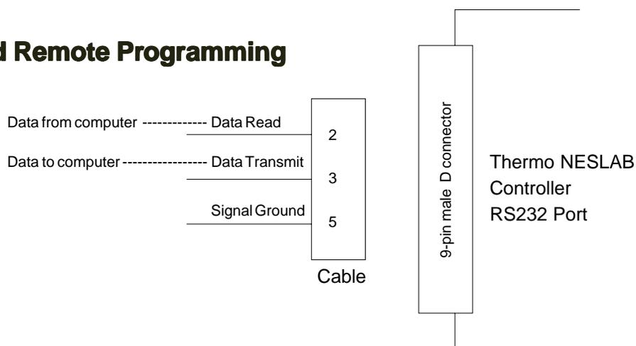
The unit can be controlled through your computer's serial port by using a standard 9-pin RS232 connection on the rear of the temperature controller. Data transmit of the serial port connects to data read (pin 2) of the bath. Data read of the serial port connects to the data transmit (pin 3) of the bath.
