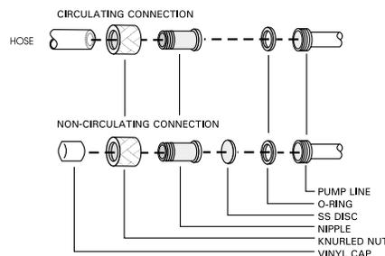
The pump lines have 1/4" male pipe threads for mating with standard plumbing fittings. For your convenience two stainless steel adapters, 1/4" female pipe thread to 3/8" O.D. serrated fitting, are provided. (To assure proper fit, they should be installed using Teflon® tape around the threads.)
