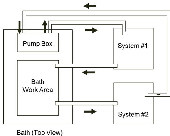
The pump can be used to circulate through two closed loop systems. Connect the shortest practical length of flexible tubing from the PUMP OUTLET to the inlet of external system #1. Connect the outlet of system #1 directly into the bath work area. Connect tubing from the bath work area to the inlet of system #2. Connect the outlet of system #2 to the PUMP INLET.
